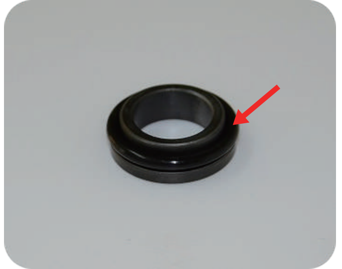
Step7: put O-ring(AS568-117) into the fixed ring
