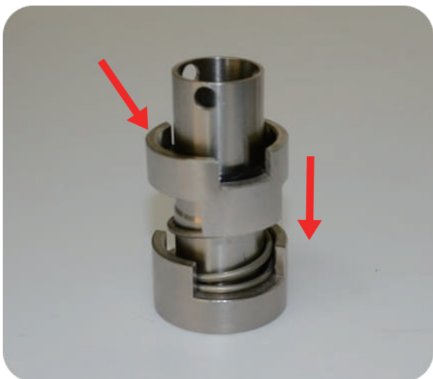
Step4: put the sheath into the shaft
