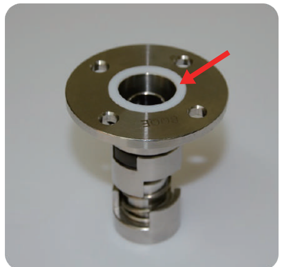
Step10: put the fixed ring on it
