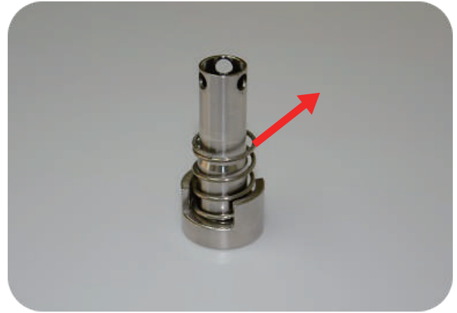
Step8: take compress spring out
