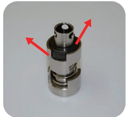
Step6: take rotation of the ring, sheath out
