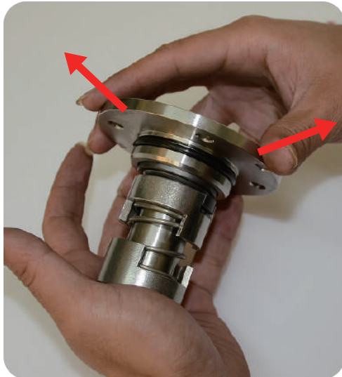
Step3: take out the set base of shaft seal
