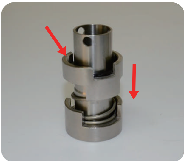
Step4: put the sheath into the shaft
