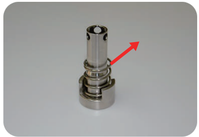
Step8: take compress spring out
