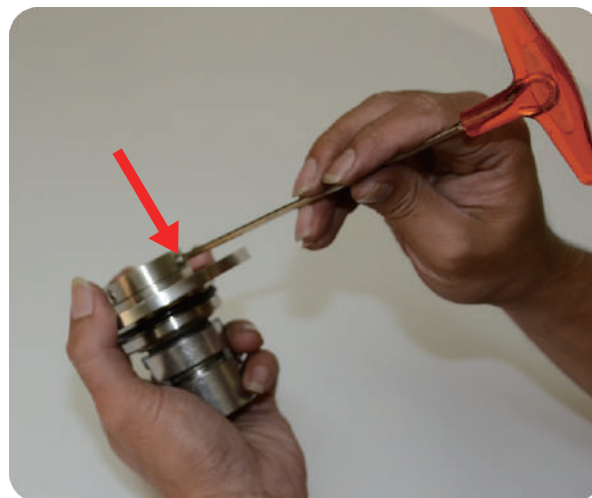
Step11: use 2.5mm hexagon wrench lock the bolt, but it cannot exceed the shaft, just not protrude the hexagon socket head
