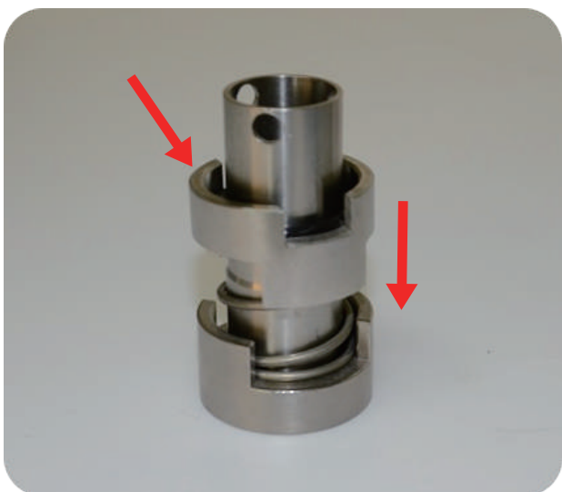
Step4: put the sheath into the shaft
