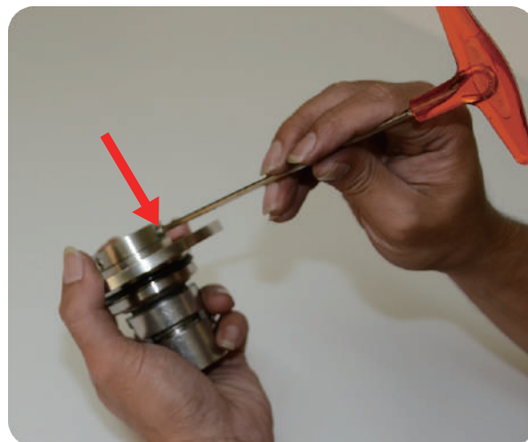
Step11: use 3mm hexagon wrench lock the bolt, but it cannot exceed the shaft, just not protrude the hexagon socket head
