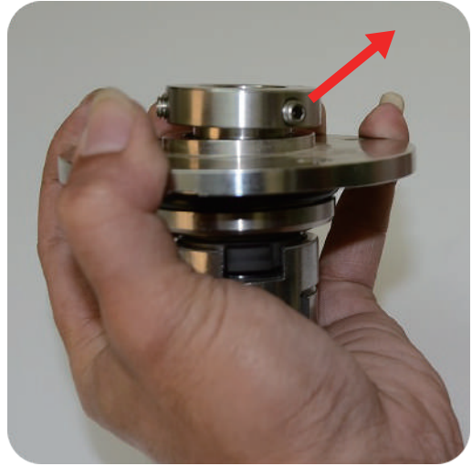
Step2: grasp the set base of shaft seal, avoid the component bounce Just loose the bolt, it's unnecessary to take hexagon socket head out
