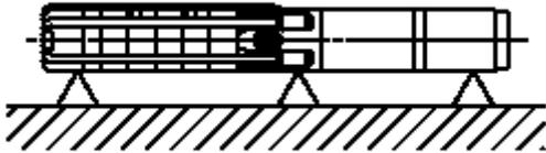
Fig. 1 Pump position during storage
