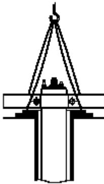
3. Lift the pump part by means of pipe clamps fitted to the extension pipe, see fig. 3.
